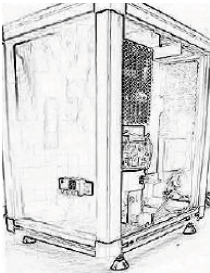
SCHEMATIC DRAWING OF APOLLO ENERGY SYSTEMS' AMMONIA CRACKER: ASSISTANCE WAS PROVIDED TO THE CLEAN AMMONIA PROJECT OF SASKATOON
