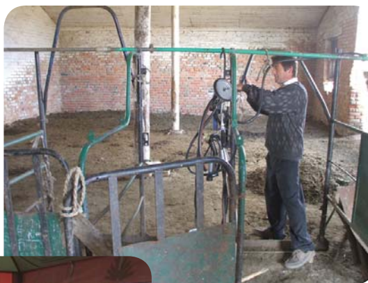
Installing new milking equipment in old state farm building
